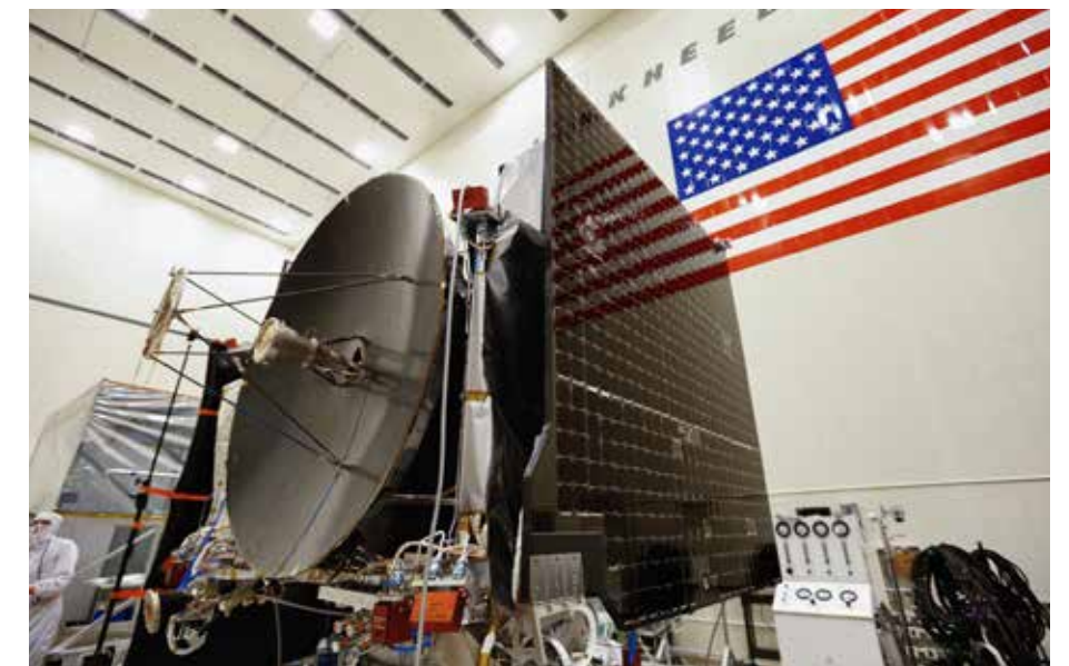
OSIRIS-REx displays its high-gain antenna and solar arrays before engineers move it from construction to environmental testing in October 2015. LOCKHEED MARTIN CORP.
