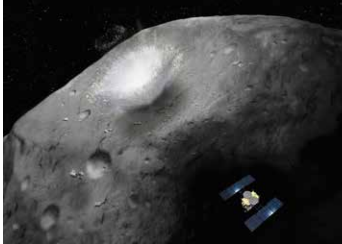
Hayabusa2 will shoot an explosive charge into asteroid Ryugu and then flee to the space rock's far side to avoid damage when it blows. The spacecraft will return to sweep up the pulverized material churned up from deep inside the asteroid's bulk. AKIHIRO IKESHITA
