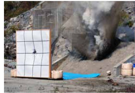
Japanese Aerospace Exploration Agency scientists successfully test Hayabusa2's Small Carry-on Impactor. They plan to use it to blow a 33-foot (10 meters) crater in asteroid Ryugu to collect samples from its interior. JAXA/NIHONKOHI
