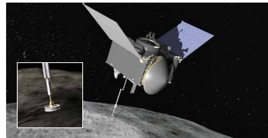
OSIRIS-REx will reach out its sample collector like a vacuum cleaner extension (inset) to gather samples from asteroid Benu's surface, possibly retrieving up to a few pounds. NASA GODDARD SPACE FLIGHT CENTER
